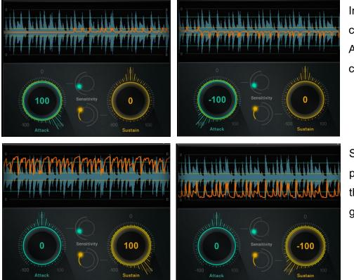
Increasing Attack Level results in a positive gain change indicator, as seen on the left. Negative Attack Level is displayed as downward gain change.
